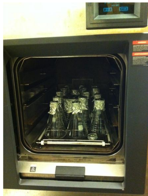
Figure 3. Autoclave for sterilization of seawater and glassware.
