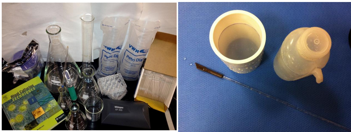
Figure 12. Necessary laboratory equipment for successful cultivation: Left: sterile vacuum filter for making stock solutions, “Algal Culturing Techniques”, various sized Erlenmeyer flasks, beaker, refractometer, thermometer, graduated cylinder, Petri dishes, multiwall plates, air pump, and Pasteur pipettes. Right: Custom filter (10-100 micron mesh), squirt bottle with sterilized seawater, and glass stir rod with rubber policeman scraper useful for
