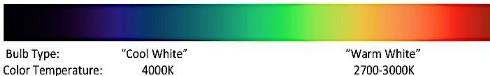
Figure 8. Fluorescent bulb color temperatures
